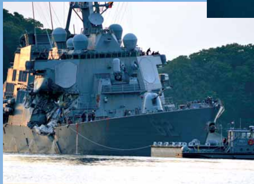
The tremendous amount of damage inflicted to the USS Fitzgerald is well-portrayed in this view of the starboard side of the destroyer. The Arleigh Burke-class guided-missile destroyer (DDG-62) was photographed on 17 June returning to Fleet Activities (FLEACT) Yokosuka following the disastrous collision with a Japanese cargo container ship that was heading out of Yokosuka, Japan. Suffering extremely severe damage, the destroyer managed to return under her own power. However, at press time the bodies of seven sailors had been recovered from the flooded portions of the damaged ship. (USN/Peter Burhart)
